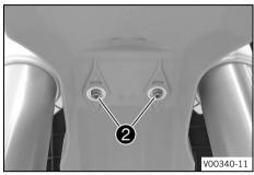
Mount and tighten screws 2.
