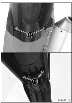
Mount and tighten screw 13 with the collar bushing.
