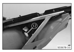
Disconnect tail light plug-in connector 12 on the wiring harness.
