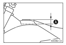
Fill the fuel tank with fuel up to level A.
