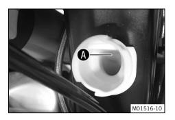
Fill the 2-stroke oil tank up to the lower edge (A) of the filler neck.
