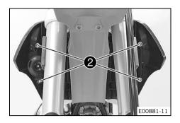
Mount and tighten screws 2 with the collar bushings.
