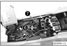
Attach starter relay 6 and fuse box 7 to the battery compartment.
