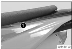
Mount and tighten screw on the left side.
