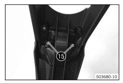
Remove screws 15 on the license plate holder and hang the tail light to the side.
