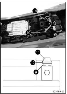
Connect positive cable to the 12-V battery.
