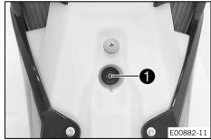
Mount and tighten screw with the rubber bushing.
