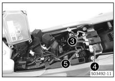
Place relays 3 and connector 4 on the battery compartment and attach the wiring harness 5.
