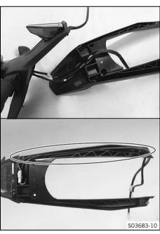
Position the tail light together with the license plate holder on the license plate bracket.
