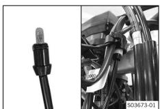
Insert the black and violet cables of bulb included in the separate enclosure into the socket and position it in the turn signal indicator lamp.
