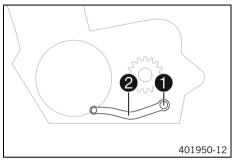
Remove screw with the washers and take off shift lever lever .
