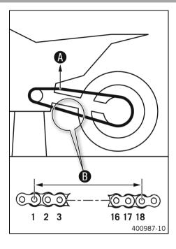
Pull on the top section of the chain with the specified weight A.
