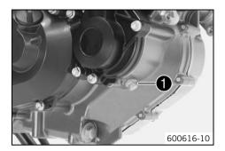
Mount and tighten screw **1** with a new seal ring. Guideline
