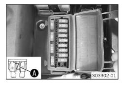
Remove the faulty fuse.
