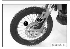
Position the left fork protector. Mount and tighten screws ①.
