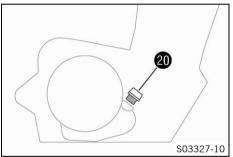
Remove filler plug with the O-ring, and fill up with engine oil.
