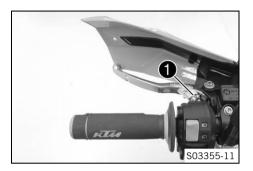
Adjust basic position of the clutch lever to your hand size by turning adjusting screw ①.
