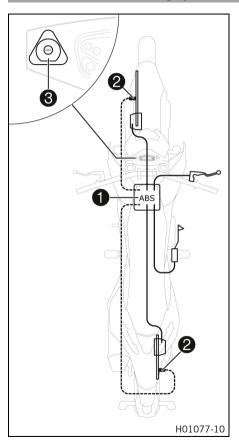
The <u>ABS</u> unit ①, which consists of a hydraulic unit, ABS control unit, and return pump, is installed under the seat. One wheel speed sensor ② is located in each case on the front and the rear wheel.
