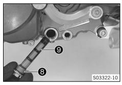
Remove screw plug **8** with oil screen **9** and the O-rings.
