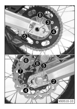
Clean and grease the thread of the wheel spindle and nut **2**.
