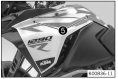
Mount and tighten screws **5**.
