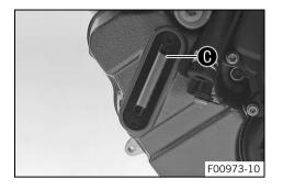
Remove the filler plug with the O-ring and add the second partial quantity up to the upper marking on the engine oil level viewer.
