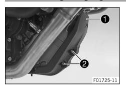
Position engine guard ①, mount screws ② with bushings and tighten.
