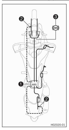
The ABS module ①, consisting of a hydraulic unit, an ABS control unit, and a return pump, is located under the seat. One wheel speed sensor ② is located in each case on the front and the rear wheel.
