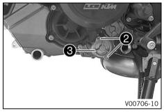
Remove screws 2. Take off oil filter cover 3 with the O-ring.
