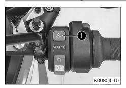
The hazard warning flasher switch 1 is fitted on the right side of the combination switch.
