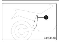
The shock absorber article number **1** is stamped on the top of the shock absorber.
