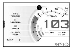
The operating state and active cruise control are shown in the **1** area of the display.
