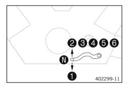
The gear positions can be seen in the figure. The idle position is between first and second gears.
