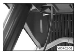
Add coolant until the coolant reaches the specified level.
