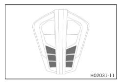
The cornering light is integrated into the main headlight.
