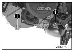
Mount and tighten oil drain plugs with the magnets, O-rings, and oil screens.
