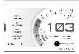
When the heated grip is switched on, the **Heated Grips** symbol appears in the **1** area of the display.
