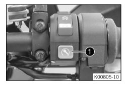
The Race-on button is fitted on the right side of the combination switch.
