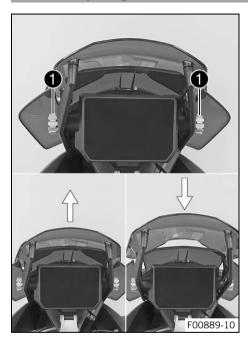
Turn the adjusting wheel 1 to bring the windshield in the required position.
