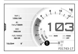
When the seat heating is switched on, the **Heated Seat** symbol appears in area **1** of the display.
