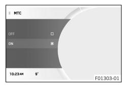
The motorcycle traction control ( $\underline{MTC}$ ) lowers the engine torque in case of loss of traction in the rear wheel. Depending on the motorcycle traction control setting, a slight slip on the rear wheel may be desirable. Example: offroad.
