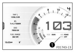
The **1** area of the display indicates whether **MTC** the system is switched on or off.
