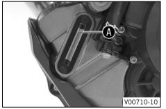
Add engine oil to upper marking (A) on the engine oil level viewer.
