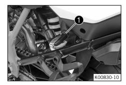
Seat lock 1 is located on the left side of the vehicle under the seat.
