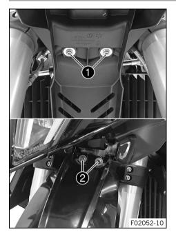
Position the front fender. Mount screws ①, but do not tighten yet.
