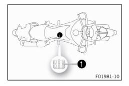
Diagnostics connector **1** is located under the battery cover.
