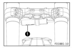
Steering damper article number **1** is embossed on the underside of the steering damper.
