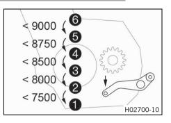
If the quickshifter + (optional) is enabled in the combination instrument, you can shift down in the speed range shown without pulling the clutch lever.
