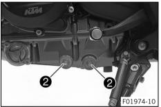
Thoroughly clean magnets (A) and oil screens (B) of the oil drain plugs.
