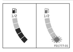
The fuel level display consists of bars. The more bars are lit, the more fuel is in the fuel tank.
