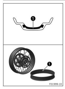
This vehicle uses a tubeless tire system in which a rim seal band **1** is used instead of the conventional tube.
