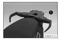
The luggage rack plate **1** is located behind the seat. The base plate of a luggage system can be mounted on the luggage rack plate (optional).
