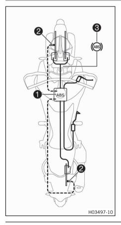
ABS module ①, which consists of a hydraulic unit, ABS control unit, and return pump, is installed under the fuel tank. One wheel speed sensor ② is located in each case on the front and the rear wheel.
