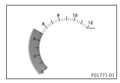
The speed is measured in revolutions per minute.
