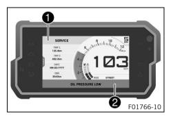
Warnings appear on the top and/or bottom edge of the display; these are marked yellow or red depending on their relevance. Yellow warnings **1** indicate a malfunction or information which requires prompt intervention or an adjustment to the riding style. Red warnings **2** indicate a malfunction or information which requires immediate intervention.
