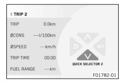
When the menu is closed, the **Quick Selector 2** display is opened by pressing the **DOWN** button. Press the **BACK** button to close the **Quick Selector 2** display.
