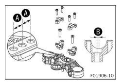
On the upper triple clamp, there are three holes at a distance of  $\mathbf{A}$  to each other.
