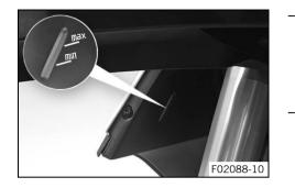
Add coolant until the coolant reaches the specified level. Guideline
