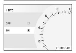
The motorcycle traction control (**MTC**) lowers the engine torque in case of loss of traction in the rear wheel.
