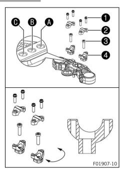
Remove screws 1. Take off the handlebar clamps 2. Position the handlebar so that screws  $\mathbf{3}$  are accessible.
