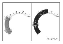
The shift warning light is integrated in the tachometer display. In the **Shift Light** submenu, the engine speed for the shift warning light can be set. The shift warning light is always active during the running-in phase (up to 1,000 km / 621 mi). The shift warning light can only be deactivated, and the values for **Lights up** and **Flashes** can only be adjusted after this. In **Lights up** the shift warning light flashes and in **Flashes** it flashes and the color changes.
