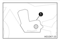
The engine number ① is stamped onto the engine case at the top.
