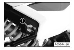
Seat lock **①** is located on the left side of the vehicle. It can be unlocked using the ignition key.
