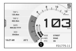
The ABS mode setting is shown in the **①** area of the display. The ABS can be configured in the **ABS** submenu.
