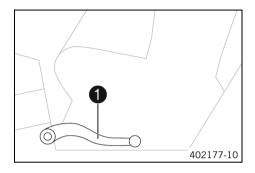
Foot brake lever **1** is located in front of the right footrest. The rear brake is activated using the foot brake lever.
