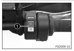
The emergency OFF switch/electric starter button **1** is located on the right side of the combination switch.
