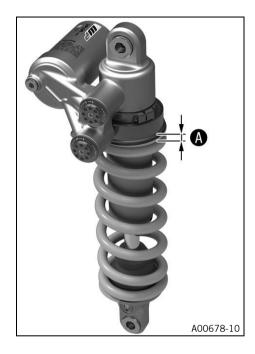
Tighten the spring to specified dimension by turning screw .
