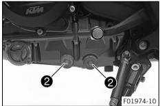
• Remove oil drain plugs **2** with the magnets, O-rings, and oil screens.
