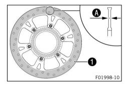
Check front and rear brake disc thickness at multiple points for the dimension **(A)**.
