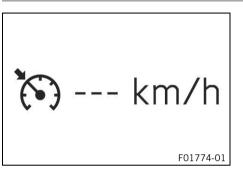
When cruise control is activated, the operating mode is shown on the combination instrument display.
