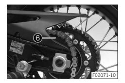
Push the rear wheel forward as far as possible. Take the chain off the rear sprocket and place it on chain sprocket guard 6.
