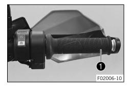
The throttle grip  $\mathbf{0}$  is fitted on the right side of the handlebar.
