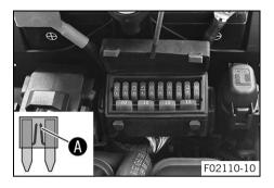
Remove the faulty fuse.
