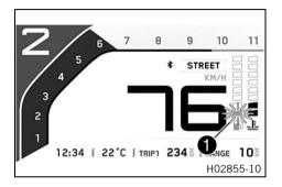
The fuel level indicator ① consists of bars. The more bars are lit, the more fuel is in the fuel tank.
