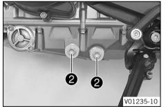
Remove oil drain plugs ② with the magnets, the O-ring, and the oil screens.
