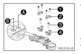
Remove screws 1. Take off the handlebar clamps 2. Position the handlebar so that screws  $\mathbf{3}$  are accessible.
