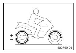
The slip adjustment is a motorcycle traction control function. The slip adjustment allows the motorcycle traction control to be tuned through nine levels to the desired characteristic map. Level 1 allows the maximum slip on the rear wheel, and level 9 the minimum.
