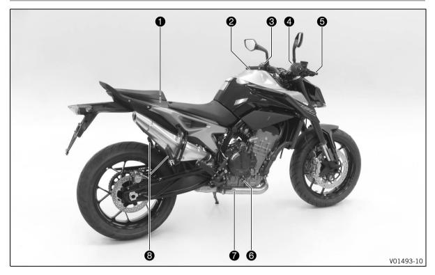
a Tool set (🕮 p. 38) 2 Fuel tank filler cap 6 Light switch (🕮 p. 30) 6 Turn signal switch (🕮 p. 31) Horn button (🕮 p. 32) 6 Emergency OFF switch/electric starter button (III p. 33) 4 6 Hand brake lever (📖 p. 28) 6 Level viewer, engine oil 1 Foot brake lever (📖 p. 41) 8 Passenger foot pegs ( p. 39)
