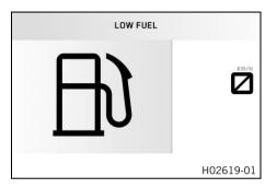
If the general warning lamp lights up among the <u>indicator lamps</u> (a) p. 48), the corresponding message appears in the display. Pressing any button confirms receipt of the information and the message is cleared.
