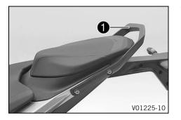
The grab handle **1** is used for maneuvering the motorcycle. If you carry a passenger, the passenger can hold onto the grab handles during the trip.
