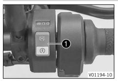
The emergency OFF switch/electric starter button ① is located on the right side of the combination switch.
