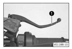
The hand brake lever  $\ensuremath{lambda}$  is located on the right side of the handlebar.
