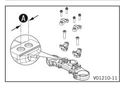
On the upper triple clamp there are two holes at a distance of **A** apart.
