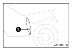
Shock absorber article number **①** is on the left side of the shock absorber.
