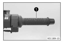
The throttle grip  $\mathbf{0}$  is fitted on the right side of the handlebar.
