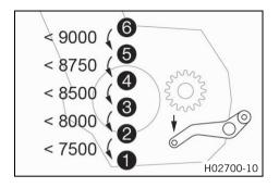
If the quickshifter + is enabled in the combination instrument, you can shift down in the speed range shown without pulling the clutch lever.
