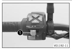
The turn signal switch **①** is fitted on the left side of the handlebar.
