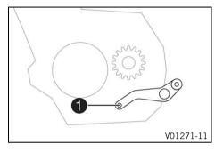
The shift lever  $\mathbf{0}$  is mounted on the left side of the engine.
