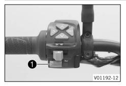
Horn button **1** is fitted on the left side of the handlebar.
