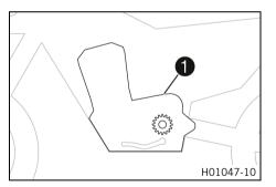
The engine number **1** is stamped onto the engine case at the top.
