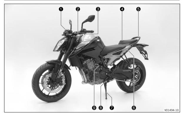
Combination instrument (IPP p. 43) a 0 Ignition and steering lock (IPP p. 34) 6 Clutch lever (🕮 p. 28) 4 Passenger seat 6 Grab handle (📖 p. 39) 6 Seat lock (📖 p. 38) 1 Side stand (🕮 p. 41) 8 Shift lever (🕮 p. 40) 0 Engine number (🕮 p. 25)
