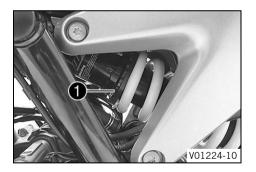
Set the spring preload by turning at the adjusting device using the hook wrench from the tool set.
