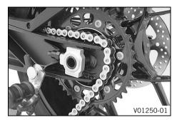
Push the rear wheel forward as far as possible. Remove the chain from the rear sprocket.
