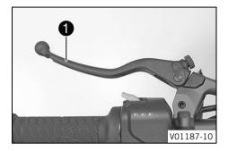
Clutch lever **1** is fitted on the handlebar on the left.
