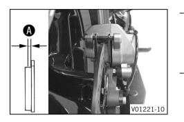
Check the brake linings for minimum thickness  $oldsymbol{A}$  .
