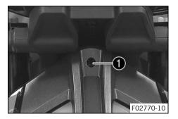
Completely unscrew adjusting screw 1.
