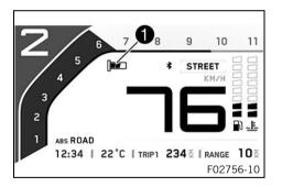
When the heated grip (optional) is switched on, the **Heated Grips** symbol appears in the **1** area of the display. The heated grip can be configured in the **Heated Grips** menu.
