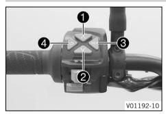
The menu buttons are fitted in the middle of the left combination switch.
