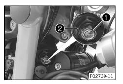
Using an open end wrench, turn adjusting screw ① clockwise all the way.
