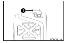
The **1** cruise control system tip switch is fitted on the left side of the combination switch.
