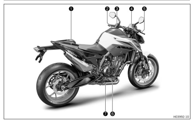
Tool set (🕮 p. 43) a 2 Fuel tank filler cap € Light switch (🕮 p. 32) € Turn signal switch (📖 p. 37) Horn button (🕮 p. 38) 6 Emergency OFF switch/electric starter button (III p. 38) 4 6 Hand brake lever (📖 p. 30) 6 Level viewer, engine oil 1 Foot brake lever (📖 p. 47)
