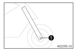
The fork part number  $\bigcirc$  is stamped on the inner side of the fork stub.
