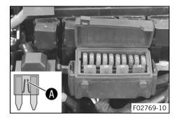
Remove the faulty fuse. \_
