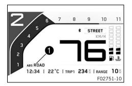
The ABS mode setting is shown in the **①** area of the display. The **ABS** can be configured in the **ABS Mode** menu.
