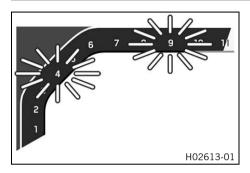
The shift warning light is integrated in the tachometer display. In the **Shift Light** menu, the engine speed for the shift warning light can be set. The shift warning light is always active during the running-in phase (up to 1,000 km / 600 mi). The shift warning light can only be deactivated, and the values for **Lights up** and **Flashes** can only be adjusted after this. The shift warning light lights up orange at **Lights up** and flashes orange at **Flashes**.
