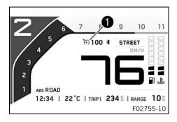
When cruise control (optional) is activated, the operating mode ① is shown on the combination instrument display. Cruise control is operated using the cruise control tip switch  $\infty$  ( $\square$  p. 33).
