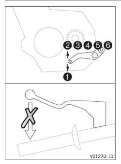
If the  $\underline{\text{quickshifter +}}$  is activated, you can shift up and down without actuating the clutch.
