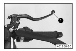
The hand brake lever **1** is located on the right side of the handlebar.
