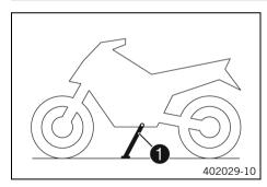
The side stand **①** is located on the left of the vehicle. The side stand is used for parking the motorcycle.
