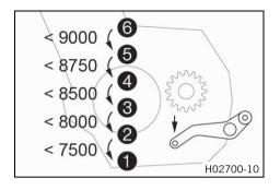
If the quickshifter + (optional) is enabled in the combination instrument, you can shift down in the speed range shown without pulling the clutch lever.
