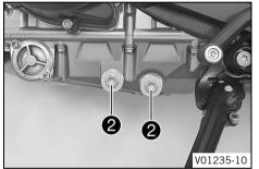
• Remove oil drain plugs **2** along with the magnets, the Orings, and the oil screens.
