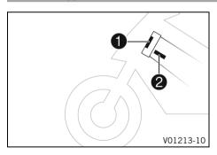
The type label **1** is located on the steering head on the left. The type label Australia **2** is located on the frame behind the steering head at the top left.
