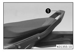
The grab handle **①** is used for maneuvering the motorcycle. If you carry a passenger, the passenger can hold onto the grab handles during the trip.
