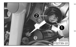
Turn adjusting screw ① clockwise with a screwdriver as far as the last perceptible click.
