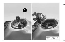
Lift cover ① of the fuel tank filler cap and insert the ignition key into the lock.
