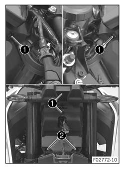
Mount and tighten screws **1**.
