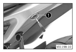
The seat lock ① is located on the left side of the vehicle. It can be locked with the ignition key.
