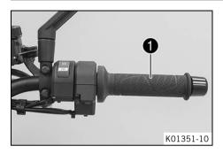
The throttle grip ① is fitted on the right side of the handlebar.
