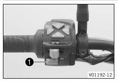
Horn button **()** is fitted on the left side of the handlebar.
