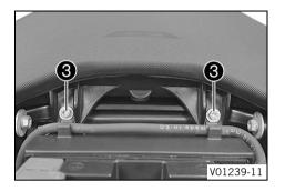
Mount and tighten screws 🚯.
