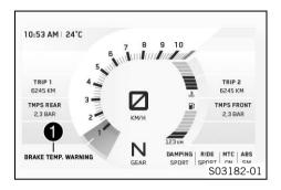
When the rear brake is used frequently and for excessively long periods, for example on long downhill stretches, the temperature of the brake system may increase.
