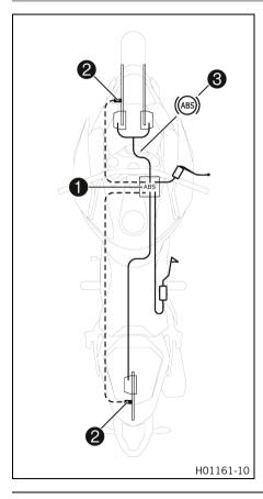
The <u>ABS</u> unit ①, which consists of a hydraulic unit, ABS control unit, and return pump, is installed on the right vehicle side below the fuel tank. One wheel speed sensor ② is located in each case on the front and the rear wheel.
