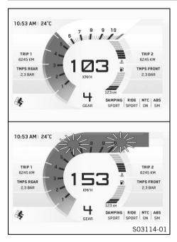
The shift warning light is integrated in the tachometer display. In the **Settings** menu under **Shift Light**, the engine speed for the shift warning light can be set. The shift warning light is always active during the running-in phase (up to 1,000 km / 621 mi). The shift warning light can only be deactivated, and the values for **Shines** and **Flashes** can only be adjusted after this. The shift warning light lights up red at **Shines** and flashes red at **Flashes**.
