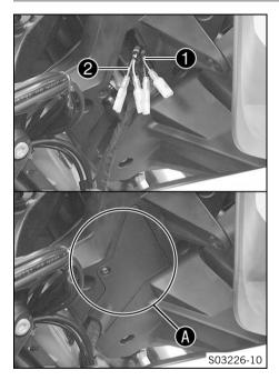
The front power supplies ACC1 **1** and ACC2 **2** are located on the right side of the instrument support behind a cover **A**.
