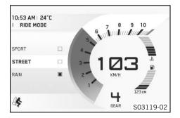
When the menu is closed,  ${\bf Quick\ Selector\ 2}$  is opened by pressing the  ${\bf DOWN}$  button.
