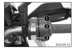
The right combination switch is fitted on the right side of the handlebar.
