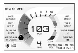
When the heated grip is activated, the **Heated Grips** symbol appears in the **①** area of the display. The heated grip can be configured in the **Motorcycle** menu under **Heated Grips**.
