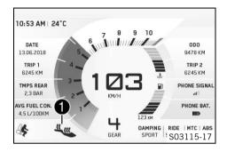
When the seat heating is activated, the **Heated Seat** symbol appears in the **①** area of the display. The seat heating can be configured in the **Motorcycle** menu under **Heated Seat**.
