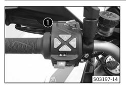
The ① cruise control system tip switch is fitted on the left side of the combination switch.
