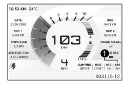
The ABS mode setting is shown in the **1** area of the display. In the menu **Motorcycle**, the ABS can be configured under **ABS**.
