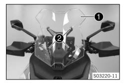
Remove screws ① with rubber bushing and windshield ②.
