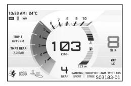
The figure shows the start screen of the combination instrument in active drive mode **TRACK** (optional) in the performance layout. In the performance layout, the standard view of the combination instrument is combined with the functions of the **TRACK** mode (optional). Only the favorites on the left are displayed. If the menu is opened, the speed is still displayed.
