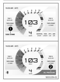
Warnings appear on the bottom edge of the display; these are marked yellow or red depending on their relevance. Yellow warnings 1 indicate errors or information which require prompt intervention or an adjustment to the riding style. Red warnings 2 indicate errors or information which require immediate intervention.
