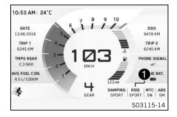
The **Ride Mode** setting is shown in area **①** of the display. The drive mode can be configured in the **Ride Mode** menu.
