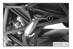
Seat lock  $\ensuremath{\textcircled{1}}$  is located on the left side of the vehicle under the seat.
