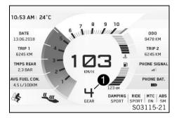
The current gear is shown in area ① of the display.
