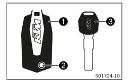
In this vehicle, the <u>RACE-ON key</u> **1** performs all the functions of the conventional ignition key.
