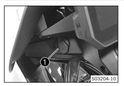
Socket **1** for electrical accessories is mounted on the left side of the instrument support.
