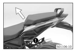
Insert the RACE-ON key or the black ignition key into seat lock
