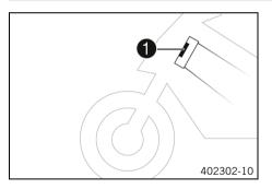
The type label **1** is located on the steering head.
