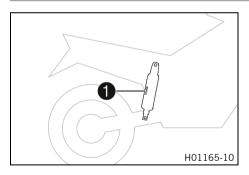
The shock absorber article number **1** is printed on a sticker on the shock absorber case under the spring.
