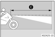
Position the vehicle perpendicular to the wall at a distance from the wall and switch on the low beam.
