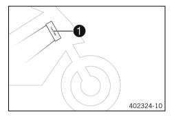
The vehicle identification number  $\ensuremath{lambda}$  is stamped on the right side of the steering head.
