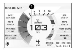
The speed is shown in area **1** of the display. The unit of speed can be configured in the **Settings** menu under **UNITS**.
