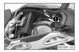
The storage compartment under the passenger seat contains tool set  $\mathbf{1}$ .
