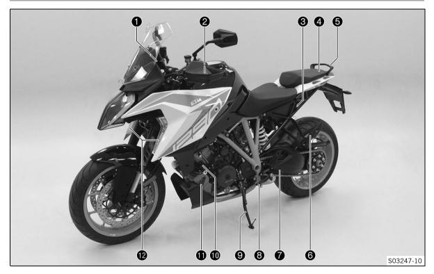
Socket for electrical accessories (IP p. 45) a 2 Clutch lever (📖 p. 30) 6 Seat lock (🕮 p. 55) 4 Tool set (🕮 p. 55) 6 Grab handle (🕮 p. 56) Passenger foot pegs (📖 p. 57) 6 1 Rider footrests 8 Shift lever (🕮 p. 58) 0 Side stand (🕮 p. 59) 10 Engine oil filler neck Ð Level viewer, engine oil 12 Cornering light (I p. 250)
