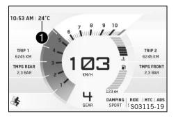
The ambient air temperature is displayed in the ① area. The units of the ambient temperature can be configured in the **Settings** menu under **Units**. The ambient air temperature is displayed in °C or °F.
