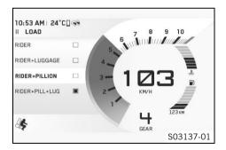
Tunings for different payloads can be selected in the **"Load"** menu. A selection can be made between one-person operation, one-person operation with luggage, two-person operation, and two-person operation with luggage.
