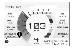
The payload setting is shown in area **1** of the display. The payload can be configured in the **Motorcycle** menu under **Load**.
