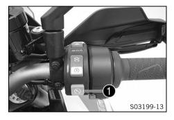
The <u>RACE-ON button</u> **(1)** is fitted on the right side of the combination switch.
