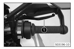
The hand brake lever  $\bigcirc$  is located on the right side of the handlebar.
