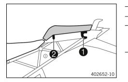
Attach hooks on the passenger seat to seat mounts 1. \_
