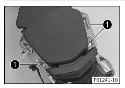
Case holders ① are located on each side of the passenger seat. A case system (optional) can be attached on the case holders. The case holders may not be loaded with more than the specified weight.
