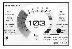
The **Damping** mode setting is shown in the **①** area of the display. The damping can be configured in the **Motorcycle** menu under **Damping**.
