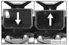
To move the combination instrument to the desired position, press combination instrument upward or downward.
