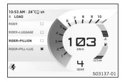
When the menu is closed,  $\ensuremath{\textbf{Quick Selector 1}}$  is opened by pressing the  $\ensuremath{\textbf{UP}}$  button.
