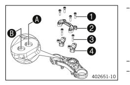
Remove screws ①. Take off handlebar clamp ②. Take off handlebar and place it to the rear.
