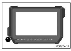
The RACE-ON indicator lamp ① can indicate errors by flashing. These are indicated up to five seconds after the RACE-ON tip switch is actuated.
