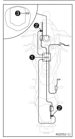
The ABS module ①, which consists of a hydraulic unit, ABS control unit, and return pump, is installed under the fuel tank. One wheel speed sensor ② is located in each case on the front and the rear wheel.
