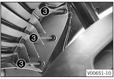
Remove expanding rivet 3.
