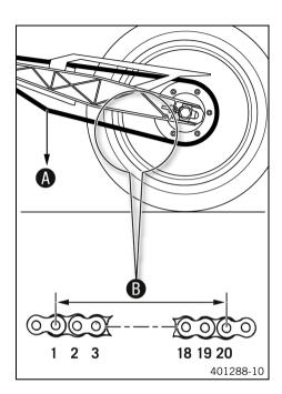
Pull on the lower chain section with the specified weight A.
