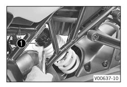
Adjust the spring preload by turning the adjusting ring using the hook wrench from the tool set.
