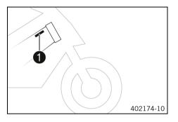
The vehicle identification number **1** is stamped on the right of the frame behind the steering head.
