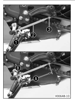
Loosen nut 1, holding threaded rod 2.
