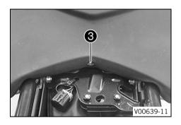
Mount and tighten screw 3 with the washer. Guideline
