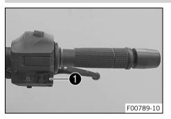
Start button 1 is fitted on the right side of the handlebar.
