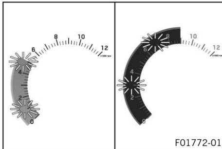
The shift warning light is integrated in the tachometer display. In the **Shift Light** menu, the engine speed for the shift warning light can be set. The shift warning light is always active during the running-in phase (up to 1,000 km / 621 mi). The shift warning light can only be deactivated, and the values for **RPM1** and **RPM2** can only be adjusted after this. In **RPM1** the shift warning light flashes and in **RPM2** it flashes and the color changes.
