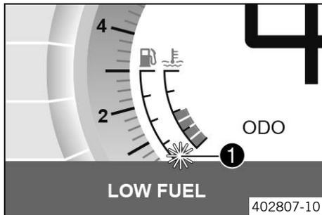
The fuel tank contents are shown in area ① of the display. The fuel level indicator consists of bars. The more bars are lit, the more fuel is in the fuel tank.
