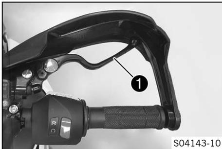
The hand brake lever ① is fitted on the right side of the handlebar.
