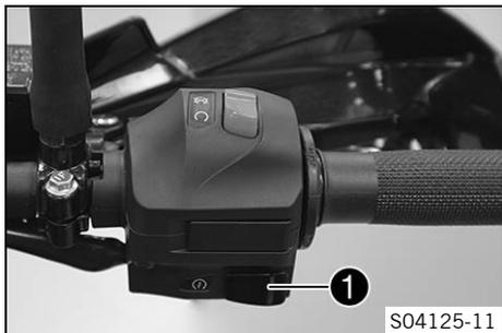
Start button ❶ is fitted on the right side of the handlebar.
