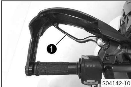
The clutch lever ① is fitted on the left side of the handlebar.
