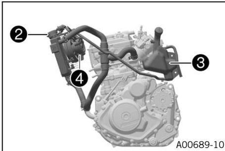
The coolant is cooled by the air stream and a radiator fan ④, which is activated at high temperature.
