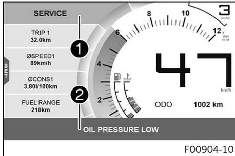
Warnings appear on the top and/or bottom edge of the display; these are marked yellow or red depending on their relevance. Yellow warnings **1** indicate malfunctions or information which require prompt intervention or an adjustment to the riding style. Red warnings **2** indicate malfunctions or information which require immediate intervention.
