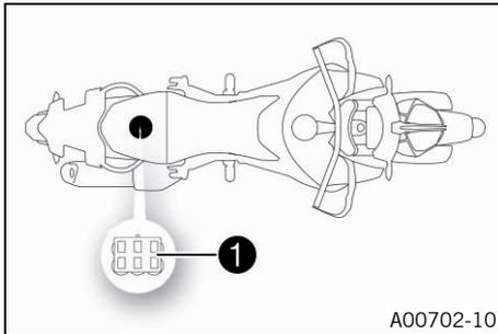
Diagnostics connector ① is located under the passenger seat.
