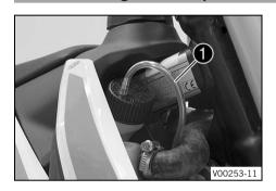
Put the oil tank cap on and turn it clockwise.
