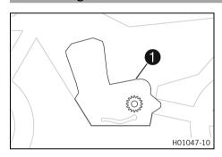
Engine number **1** is located on the left side of the engine over the engine sprocket.
