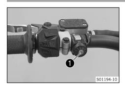
Switch-off button **1** is fitted on the left side of the handlebar. **Possible states**
