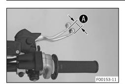
Push the hand brake lever forward and check free travel **A**.
