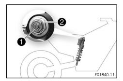
Turn adjusting screw all the way clockwise with a socket wrench.
