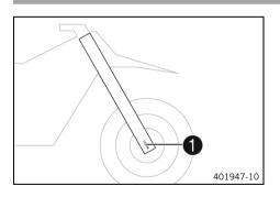
The fork article number  $\ensuremath{\mathbf{1}}$  is stamped on the inside of the axle clamp.
