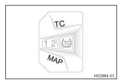
Press and hold the MAP and TC buttons simultaneously.
