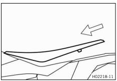
Mount the front of the seat on the collar bushing of the fuel tank, lower the seat at the rear, and push the seat forward.
