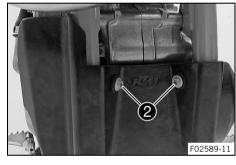
Mount and tighten screws 2.
