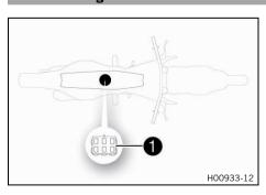
Diagnostics connector 1 is located under the seat.
