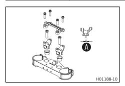
The holes on the handlebar supports are placed at a distance of  $oldsymbol{\mathbb{A}}$  from the center.
