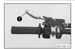
The clutch lever **1** is fitted on the left side of the handlebar. The clutch is hydraulically operated and self-adjusting.
