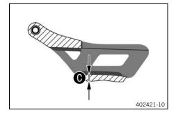
Check the chain guide with a slide gauge for dimension ①.
