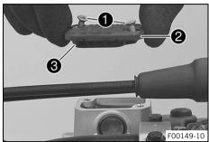
Position cover **2** with membrane **3**. Mount and tighten screws 1.
