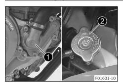
Water pump 1 in the engine circulates the coolant.
