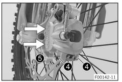
Manually press the brake caliper toward the brake disc to push back the brake pistons. Ensure that brake fluid does not flow out of the brake fluid reservoir, if necessary extract excess.
