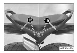
Position grab handle and mount and tighten screws **15**. Guideline
