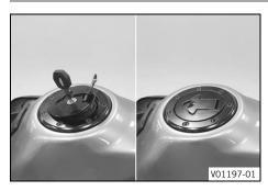
Fold down the fuel tank filler cap.
