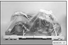
Remove the adhesive tape in the upper area of the motorcycle.
