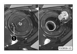
Lift cover **①** of the fuel tank filler cap and insert the ignition key into the lock.
