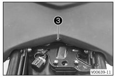
Mount and tighten screw ③ with the washer.
