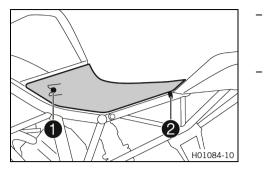
Attach recesses **①** on the front rider's seat to the fuel tank, push the front rider's seat forward, and lower at the rear.
