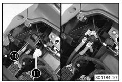
Carefully loosen and remove the tension belts around the fork legs.
