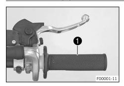
Throttle grip **1** is fitted on the right side of the handlebar.
