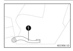
Foot brake lever **1** is located in front of the right footrest. The foot brake lever is used to activate the rear brake.
