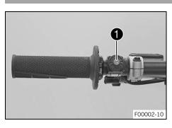
Switch-off button 1 is fitted on the left side of the handlebar.
