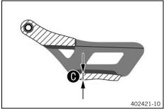
Check the chain guide with a slide gage for dimension **()**.
