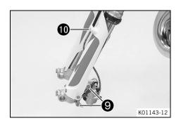
Position the brake caliper. Mount and tighten screws **9**.
