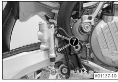
Remove screws 7 and pull foot brake cylinder off the push
