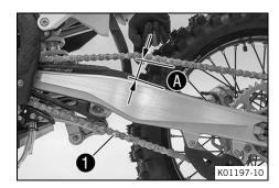
Pull the chain at the end of the chain sliding piece upward to measure chain tension A.
