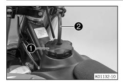
Mount fuel tank filler cap 1 and turn it clockwise until the fuel tank is tightly closed.
