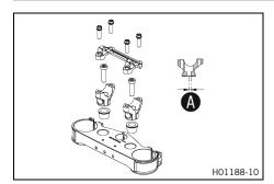
The holes on the handlebar supports are placed at a distance of  $\bf A$  from the center.
