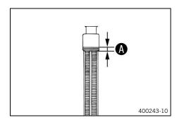
Pour coolant in up to measurement above the radiator fins.
