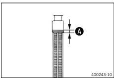
Pour coolant in up to measurement **A** above the radiator fins.
