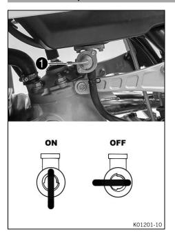
The fuel tap is on the left side of the fuel tank.
