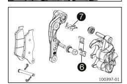
Check that spring plate 6 in the brake caliper and sliding plate 7 in the brake caliper bracket are seated correctly.
