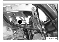
Choke ① is fitted on the left side of the carburetor.
