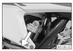
Remove the shock absorber carefully at the bottom.
