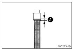
Pour coolant in up to measurement above the radiator fins.
