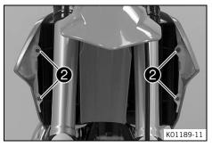
Mount and tighten screws 2.
