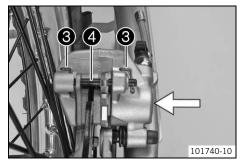
Manually press the brake caliper toward the brake disc to push back the brake piston. Ensure that brake fluid does not flow out of the brake fluid reservoir, if necessary extract excess.
