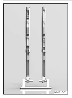
Air suspension **WP Suspension XACT 5448** is used in the fork. In this system, suspension is located in the left fork leg and damping in the right fork leg.
