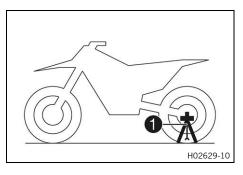
The holder for the plug-in stand **1** is the left side of the wheel spindle.
