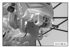
Insert the new brake linings, insert pin, and mount cotter pins.
