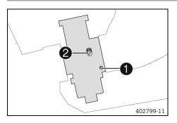
Screw in idle air adjusting screw all the way and turn it to the specified basic setting.
