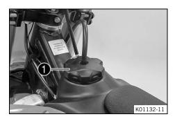
Turn fuel tank filler cap 1 counterclockwise and lift it off.
