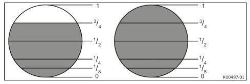
When the throttle slide is 3/4 open, the influence of the main jet is greatest. The clip position and the idling jet have only minimal influence.
