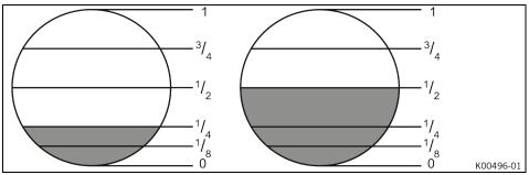
When the throttle slide is 1/4 open, the idling jet and the clip position have the greatest influence. The influence of the first cylindrical part of the needle is less.
