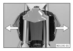
Pull both spoilers laterally off the radiator and take off the fuel tank upwards.
