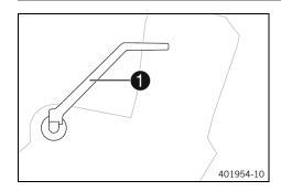
Kick starter lever **1** is fitted on the right side of the engine. The kick starter lever can be swiveled.
