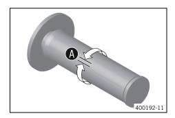
Turn barrel adjuster **2** so that there is play **A** in the throttle cable at the throttle grip.
