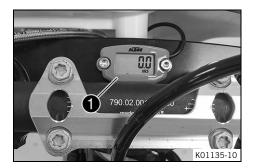
The service hour counter 1 is fitted in front of the handlebar. It shows the total number of service hours of the engine. The service hour counter begins counting when the engine is started and stops when the engine is switched off.
