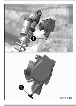
The cold start button **()** is fitted to the bottom of the throttle valve body.
