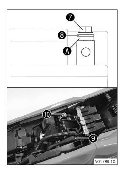
Connect the positive cable to the 12-V battery. Guideline
