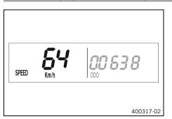
The current speed is displayed in the **SPEED** display mode. The current speed can be displayed in **Km/h** or **Mph**.
