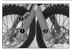
Position the fork protector on the left fork leg. Mount and tighten screws **1**.
