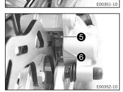
Check that spring plate **(5)** in the brake caliper and sliding plate **(6)** in the brake caliper bracket are seated properly.
