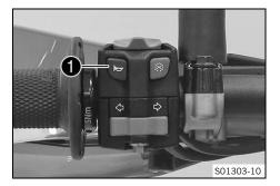
Horn button **1** is fitted on the left side of the handlebar. **Possible states**
