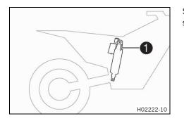
Shock absorber article number **1** is stamped on the top of the shock absorber above the adjusting ring towards the engine side.
