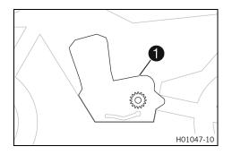
Engine number **1** is embossed on the left side of the engine over the engine sprocket.
