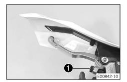
Adjust the basic position of the clutch lever to your hand size by turning adjusting screw **1**.
