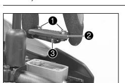
Move the clutch fluid reservoir mounted on the handlebar to a horizontal position.
