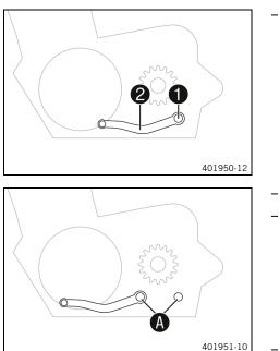
Remove screw **①** with the washers and take off shift lever 2.
