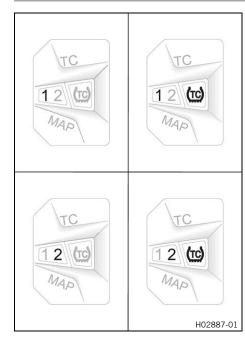
The combination switch is fitted on the left side of the handlebar. **Possible states**
