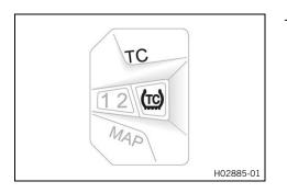
Press button **TC** to switch the traction control on or off. Guideline
