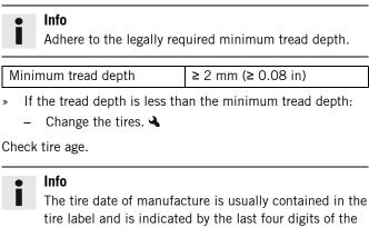
tire label and is indicated by the last four digits of the **DOT** number. The first two digits indicate the week of manufacture and the last two digits the year of manufacture.
