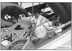
Insert the new brake linings, insert the pin, and mount the cotter pins.
