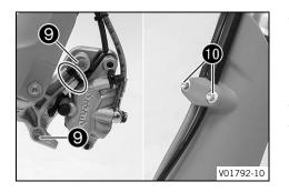
Position the brake caliper, and mount and tighten screws **(9)**. Guideline
