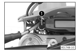
The light switch **1** is attached next to the combination instrument on the left.
