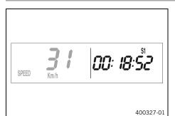
**S1** (Stop watch 1) shows the riding time based on **TR1** and continues running as soon as an impulse arrives from the wheel speed sensor.
