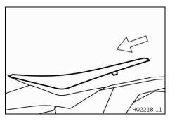
Mount the front of the seat on the collar bushings of the fuel tank, lower the seat at the rear, and push the seat forward.
