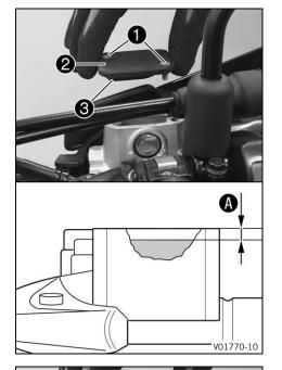
Correct the brake fluid level to level A.
