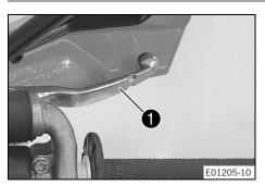
The hand brake lever ① is fitted on the right side of the handlebar. The hand brake lever is used to activate the front brake.
