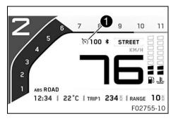
When cruise control (optional) is activated, the operating mode is shown on the combination instrument display.
