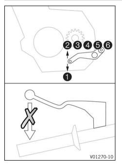
If the <u>quickshifter +</u> is activated, you can shift up and down without actuating the clutch.
