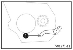
The shift lever **1** is mounted on the left side of the engine.
