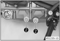
Remove oil drain plugs 2 along with the magnets, the O-rings, and the oil screens.
