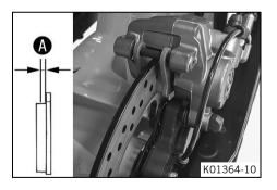
Check the brake linings for minimum thickness **A**.
