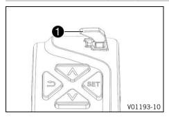
The ① cruise control system tip switch is fitted on the left side of the combination switch.
