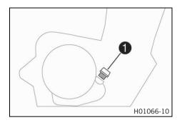
Mount and tighten filler plug with the O-ring.
