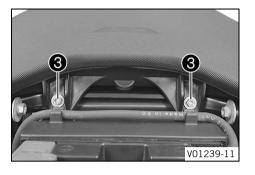
Mount and tighten screws 3.
