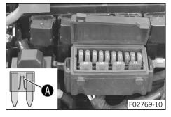
Remove the faulty fuse.
