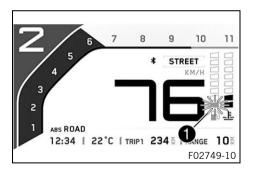
The fuel level indicator **1** consists of bars. The more bars are lit, the more fuel is in the fuel tank.
