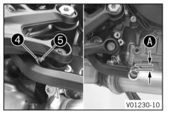
Loosen nut 4 and turn screw 5 correspondingly until the free travel A is present. If necessary, adjust the basic position of the foot brake lever.
