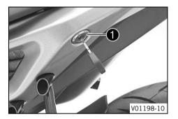
The seat lock is located on the left side of the vehicle. It can be locked with the ignition key.
