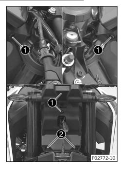
Mount and tighten screws 1.
