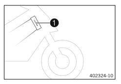
The vehicle identification number **1** is stamped on the right side of the steering head.
