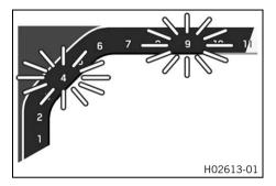
The shift warning light is integrated in the tachometer display. In the **Shift Light** menu, the engine speed for the shift warning light can be set. The shift warning light is always active during the running-in phase (up to 1,000~km / 600~mi). The shift warning light can only be deactivated, and the values for **Lights up** and **Flashes** can only be adjusted after this. The shift warning light lights up orange at **Lights up** and flashes orange at **Flashes**.
