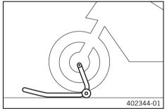
Move the handlebar to the straight-ahead position. Align the lifting gear at the front with the adapters to the fork legs.
