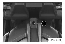
Completely unscrew adjusting screw 1.
