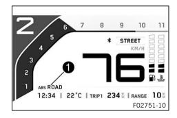
The ABS mode setting is shown in the **1** area of the display. The **ABS** can be configured in the **ABS Mode** menu.
