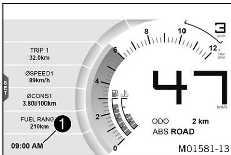
The time is shown in area **1** of the display. The time is displayed in 24 hour format in all languages except for EN-US. The time is displayed in 12 hour format if the language is set to EN-US. The time can be configured in the **Clock/Date** menu.
