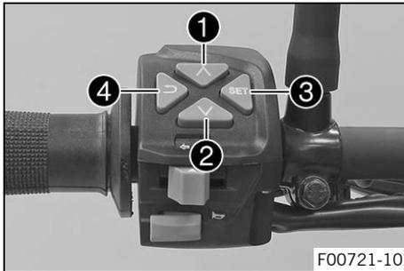
The menu buttons are fitted in the middle of the left combination switch.
