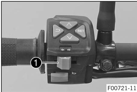
Turn signal switch ① is fitted on the left side of the handlebar.
