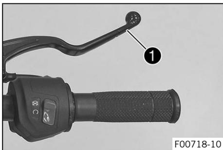
The hand brake lever **1** is fitted on the right side of the handlebar.
