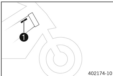
The type label ❶ is on the right of the frame behind the steering head.
