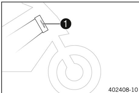
The vehicle identification number ❶ is stamped on the right side of the steering head.
