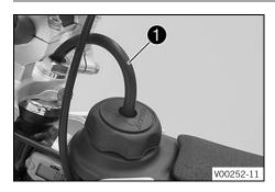
Mount the fuel tank filler cap and turn it clockwise until the fuel tank is tightly closed.
