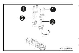
Remove screws **1**. Take off the handlebar clamps. Remove the handlebar and lay it to one side.
