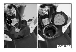
Press release button ①, turn the fuel tank filler cap counterclockwise, and lift it off.
