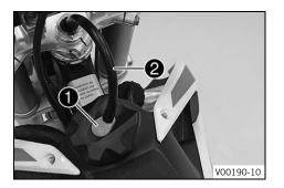
Mount the fuel tank filler cap and turn it clockwise until release button **1** engages.
