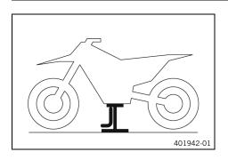
Raise the motorcycle at the frame underneath the engine.
