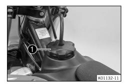
Turn fuel tank filler cap ① counterclockwise and lift it off.
