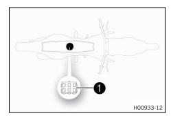
Diagnostics connector 1 is located under the seat.
