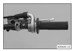
Position the controls on the right half of the handlebar.
