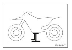
Remove the plug-in stand and lift up the motorcycle by the frame underneath the engine.
