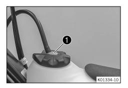
Press release button ①, turn the fuel tank filler cap counterclockwise, and lift it off.
