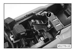
3.14 Installing the 12-V battery
