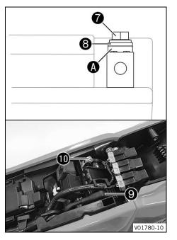
Connect the positive cable to the 12-V battery. Guideline
