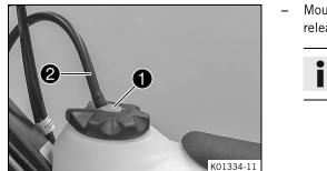
Mount the fuel tank filler cap and turn it clockwise until release button ① engages.
