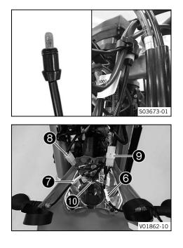
Insert the black and violet cables of bulb included in the separate enclosure into the socket and position it in the turn signal indicator lamp.
