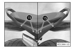
Position grab handle and mount and tighten screws 15.
