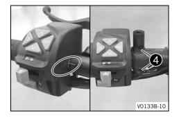
Align the controls of the left handlebar half with the markings on the handlebar. Tighten the screws.
