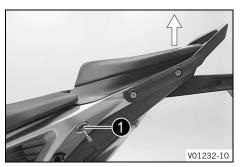
– Insert the ignition key in seat lock ① and turn it clockwise.
