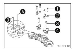
Remove screws **1**. Take off the handlebar clamps **2**. Position the handlebar so that screws **3** are accessible.
