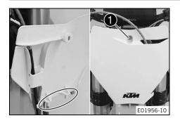
Position the brake line in holders on the start number plate.
