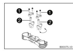
Remove screws ①. Take off the handlebar clamps. Remove the handlebar and lay it to one side.
