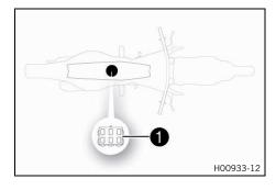
The diagnostics connector **1** is located under the seat below the EFI control unit.
