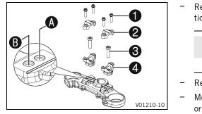
Remove screws ①. Take off the handlebar clamps ②. Position the handlebar so that screws ③ are accessible.
