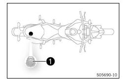
Diagnostics connector 1 is located under the passenger seat.
