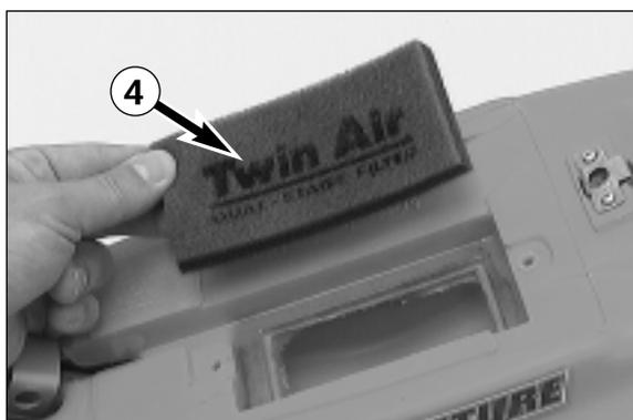
Thoroughly wash the foam filter in special cleaning fluid and allow it to dry well. Only press out the filter, do not wring it out under any circumstances. Oil the dry foam filter with a high-grade filter oil. Also clean the air filter box. Check carburetor collar for damage and that it is filled correctly.
