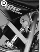
Figures C and D show the fork and shock absorber positions for a high seat position. Fork tubes are plane with top of upper fork stabilizer. (Screw cap (Aluminium) protrudes top of upper fork stabilizer)
