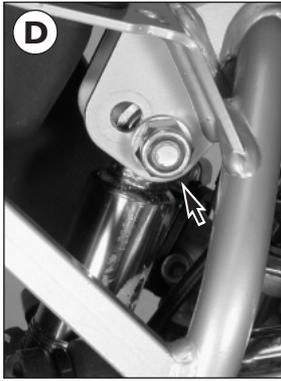
Figures C and D show the fork and shock absorber positions for a high seat position. Fork tubes are plane with top of upper fork stabilizer. (Screw cap (Aluminium) protrudes top of upper fork stabilizer)
