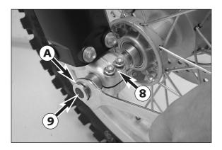
Insert the front wheel in the fork and adjust to the right position.
