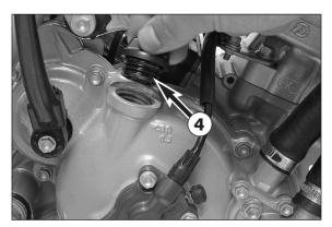
Remove the filler plug **4** and add 0.30 l gear oil 20W30 (i.ex. Shell Advance Ultra 4).
