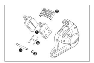
Insert the new brake pads 1 into the brake caliper, position the leaf spring **6**, and secure it with the bolt **6**. By tapping on the bolt, drive it into the brake caliper up to the stop. Reattach locking ring 3 and cover 2.
