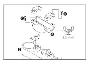
For this purpose, remove screws 6 of the handlebar clamps and screws 6 of the handlebar support. Position handlebar support, and tighten screws 6 to 40 Nm (30 ft.lbs). Mount handlebar and handlebar clamps, and tighten screws 6 to 20 Nm (15 ft.lbs). The gap between handlebar support and handlebar clamps is to be of equal size in the front and in the rear.
