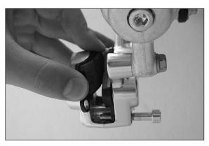
Mount the right brake shoe and fix with screw. Mount the left brake shoe and tighten the screw to 10 Nm. Mount the lock washer. Align brake shoes, mount front wheel (see chapter: Mounting the front wheel).
