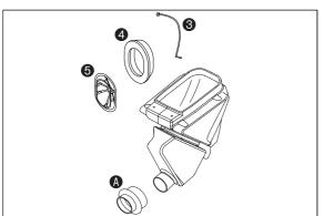
Thoroughly wash the foam filter in special cleaning fluid and allow to dry well. Only press out the filter, do not wring out under any circumstances. Oil the dry foam filter with a high grade filter oil. Also clean the air filter box. Check carburettor collar **a** for damage and that it is fitted correctly.
