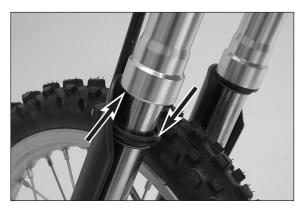
Clean dust-protection bellows, outer tubes, and fork tubes thoroughly, and oil them thoroughly with silicone spray or engine oil. Then, push dust-protection bellows into the outer tubes by hand.
