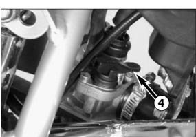
The choke lever 4 is located on the right side of the carburetor. When pulling the choke lever fully towards the top, a bore is opened in the carburetor. Through this bore the engine can take in additional fuel. This results in a rich fuel-air mixture that is needed for a cold start.
