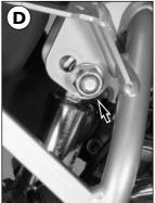
Figures C and D show the fork and shock absorber positions for a high seat position. Fork tubes are plane with top of top triple clamp. (Bold cap (Aluminium) protrudes from the top of the top triple clamp)
