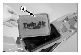
Thoroughly wash the foam filter in special cleaning fluid and allow it to dry well. Only press out the filter, do not wring it out under any circumstances. Oil the dry foam filter with a high-grade filter oil. Also clean the air filter box. Check carburetor collar for damage and that it is filled correctly. Insert the air filter in the opening and fasten it with the filter holder. Then mount the seat.
