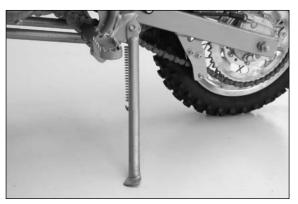
**Side stand**Use your foot to swing the side stand forwards to the stop. Make sure it rests securely on solid ground.
