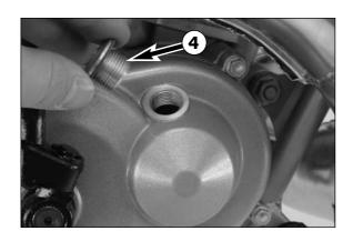
Remove stopper **4** and fill in 0.15 liters of automatic gear oil (Shell Donax TA). Mount the stopper and check the engine for tightness.
