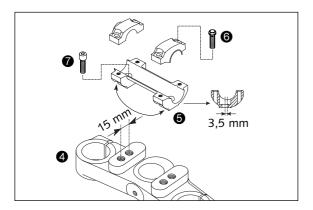
For this purpose, remove screws **3** of the handlebar clamps and screws **4** of the handlebar support. Position handlebar support, and tighten screws **4** to 40 Nm. Mount handlebar and handlebar clamps, and tighten screws **5** to 20 Nm. The gap between the handlebar support and handlebar clamps should be the same size in the front and in the rear.
