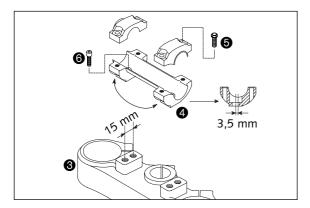
For this purpose, remove screws **6** of the handlebar clamps and screws **6** of the handlebar support. Position handlebar support, and tighten screws **6** to 40 Nm. Mount handlebar and handlebar clamps, and tighten screws **6** to 20 Nm. The gap between the handlebar support and handlebar clamps should be the same size in the front and in the rear.
