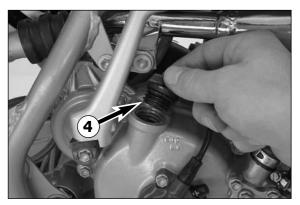
Remove the filler plug **4** and add 0.30 I gear oil 20W30 (e.g. Shell Advance Ultra 4). Mount the filler plug and check the engine for leaks.
