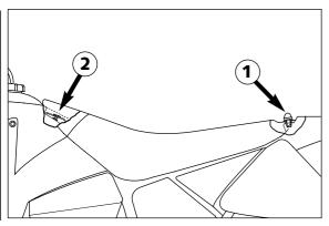
To mount the seat, position seat on the fixing screw ② and tank, push forward and fix with the quick release.
