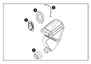
Mount the air filter **3** on the filter support **5**. Grease the front side of the filter to improve the seal. Mount the air filter and the filter support in the filter box. Make sure they are centered, and lock into place with the filter holder **3**.
