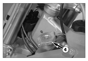
A mixture of 40% antifreeze liquid and 60% water is used as coolant. However, the antifreeze protection must be at least -25° C (-13° F). This mixture offers antifreeze protection but also good corrosion protection and should therefore not be replaced by pure water.
