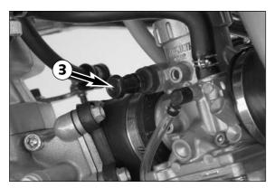
The choke button  $\ \ \mathbf 3 \$  is located on the left side of the carburetor. Pulling the choke button  $\ \ \mathbf 3 \$  all the way out opens a bore in the carburetor through which the engine can take in additional fuel, thus achieving the "rich" fuel air mixture needed for cold starting.
