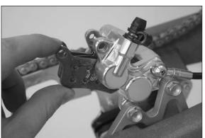
Press both brake shoes into the brake caliper and fix with bolt 2. Mount the locks **1**.
