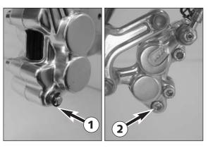
Remove the lock washer 1 from the screw as well as fixing screw 2 and take the brake shoes out of the brake caliper. Clean brake caliper thoroughly with compressed air.
