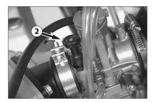
The choke button ② is located on the left side of the carburetor. Pulling the choke button 2 all the way out opens a bore in the carburetor through which the engine can take in additional fuel, thus achieving the "rich" fuel air mixture needed for cold starting.
