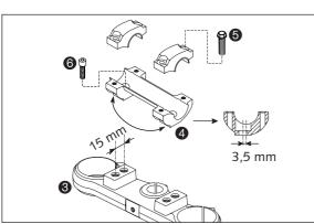
For this purpose, remove screws **6** of the handlebar clamps and screws **6** of the handlebar support. Position handlebar support, and tighten screws **6** to 40 Nm. Mount handlebar and handlebar clamps, and tighten screws **6** to 20 Nm. The gap between the handlebar support and handlebar clamps should be the same size in the front and in the rear.
