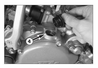
Remove the filler plug **4** and add 0.35 I gear oil (e.g. Motorex Topspeed 4T 15W50). Mount the filler plug and check the engine for leaks.
