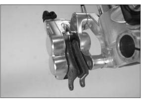
Mount both brake shoes and fasten with the fixing screw. Tighten the fixing screw to 10 Nm. Mount the lock washer. Align the brake shoes, mount the front wheel (see chapter "Mounting the front wheel").
