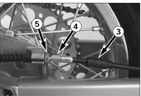
Before adjusting the brake control cable push back the protection cover ③. Undo the counter nut ⑤ and twist the adjustment screw ④ until the desired adjustment is achieved. After the adjustment process retighten the counter nut ⑤ and mount protection cover.
