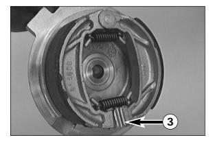
Slightly roughen the new brake shoes with an abrasive cloth and hook both springs into the brake shoes.
