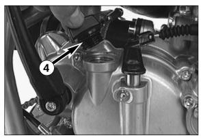
Remove the filler plug 4 and add 0.30 I engine oil 10W40 (e.g. Shell Advance Ultra 4). Mount the filler plug and check the engine for leaks.
