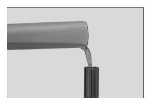
Fill the fork tubes with new fork oil (SAE 7.5)
