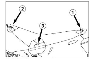
When installing the seat, be sure to insert the rear portion of the seat into the metal clasp  $\Theta$ .
