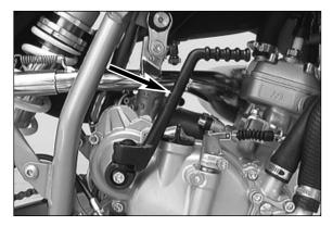
**Kickstarter** The kickstarter is mounted on the right side of the engine. Its upper part can be swivelled.
