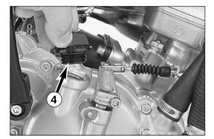
Remove the filler plug 4 and add 0.30 I engine oil 10W40 (e.g. Shell Advance Ultra 4). Mount the filler plug and check the engine for leaks.
