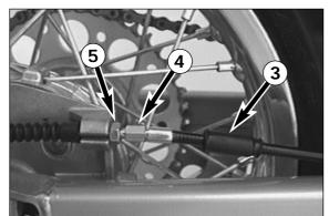
Before adjusting the brake control cable push back the protection cover 3. Undo the counter nut 3 and twist the adjustment screw 3 until the desired adjustment is achieved. After the adjustment process retighten the counter nut 3 and mount protection cover.
