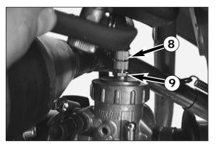
To adjust the throttle cable undo the counter nut **9** at the carburetor and twist the adjustment screw **9** until the desired adjustment is achieved. After the adjustment process retighten the counter nut **9** and make sure the protection cover is properly put back into place.
