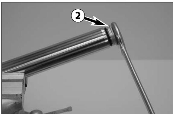
Clamp the fork leg into a vise (use protective jaws) and remove the plugs ❷.
