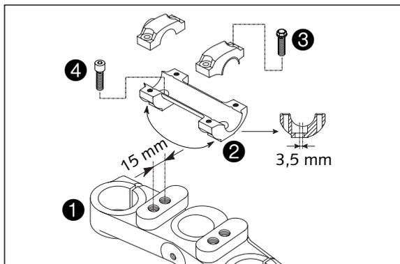
For this purpose, remove screws ③ of the handlebar clamps and screws ④ of the handlebar support. Position handlebar support, and tighten screws ④ to 40 Nm. Mount handlebar and handlebar clamps, and tighten screws ③ to 20 Nm. The gap between the handlebar support and handlebar clamps should be the same size in the front and in the rear.
