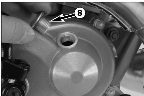
Remove stopper ⑧ and fill in 0.15 liters of automatic gear oil (Motorex ATF Super). Mount the stopper and check the engine for tightness.
