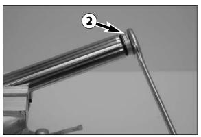
Clamp the fork leg into a vise (use protective jaws) and remove the plugs  $oldsymbol{2}$ .
