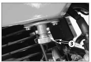
The fuel tap **3** is located at the front of the motorcycle on the left side of the tank.
