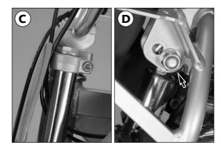
Figures C and D show the fork and shock absorber positions for a high seat position. Fork tubes are plane with top of top triple clamp. (Bold cap (Aluminium) protrudes from the top of the top triple clamp)
