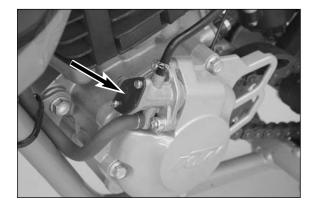
The oil pump is mounted on the ignition cover and is powered by the crankshaft.
