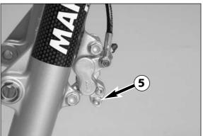
Mount the right brake shoe and fix with screw. Mount the left brake shoe and tighten the screw to 6 Nm. Mount the lock washer. Align brake shoes, mount front wheel (see chapter: Mounting the front wheel).
