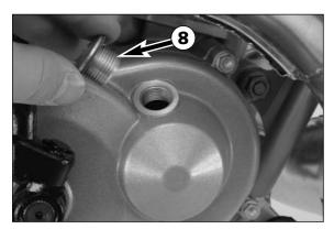
Remove stopper **3** and fill in 0.15 liters of automatic gear oil (Motorex ATF Super). Mount the stopper and check the engine for tightness.
