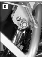
Figures C and D show the fork and shock absorber positions for a high seat position. Fork tubes are plane with top of top triple clamp. (Bold cap (Aluminium) protrudes from the top of the top triple clamp)
