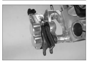
Mount the right brake shoe and fix with screw. Mount the left brake shoe and tighten the screw to 4 Nm. Mount the lock washer. Align brake shoes, mount front wheel (see chapter: Mounting the front wheel).
