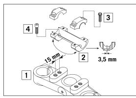
For this purpose, remove screws [3] of the handlebar clamps and screws [4] of the handlebar support. Position handlebar support, and tighten screws [4] to 40 Nm. Mount handlebar and handlebar clamps, and tighten screws [3] to 20 Nm. The gap between the handlebar support and handlebar clamps should be the same size in the front and in the rear.
