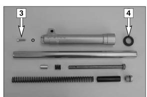
Thoroughly clean all parts and check for wear. Grease gaskets and springs and reassemble the telescopic fork. Tighten the screws at the underside of the slider tubes to 30 Nm. Fill in fork oil and assemble the fork (see below). Insert the fork legs into the triple clamps (projection as previously noted) and tighten the clamp screws to 20 Nm (top) and 10 Nm (bottom). Mount the front wheel (see chapter: mounting the front wheel).
