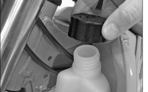
7 OIL TANK (50 MINI ADVENTURE) Check the oil level in the tank. A shortage of two-stroke engine oil will lead to engine damage.
