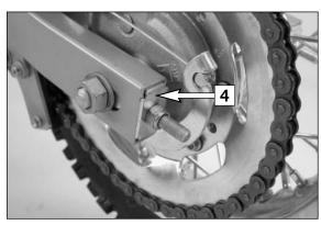
To mount the wheel reverse the procedure described above. Always hook the brake backing plate into the swing arm support. Before tightening the hexagon nut of the wheel spindle, ensure that the supporting plates [4] are resting against the swing arm. Additionally, check that
