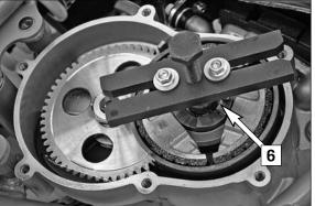
Completely remove the centrifugal clutch, bearings and spacing washers from the crankshaft.
