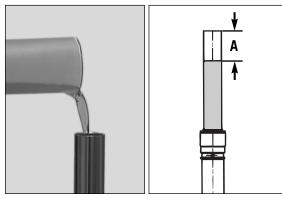
Pour 170 cm<sup>3</sup> SAE 7.5 fork oil into each fork tube. Slide the fork tube all the way into the slider tube. Adjust the air-chamber length **A** to 110 mm (4.5 in) by extracting or adding fork oil. Insert springs and pretensioning sleeves into the fork tube. Check O-rings, grease and mount plugs. Mount fork legs and front wheel (see above). Mount brake control cable and brake cable guide. Adjust the cable control on the front brake.
