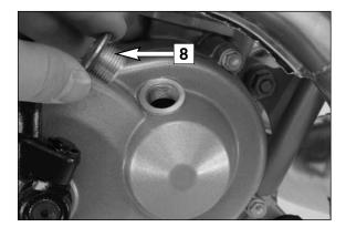
Remove stopper **[8]** and fill in 0.15 liters of automatic gear oil (Motorex ATF Super). Mount the stopper and check the engine for tightness.
