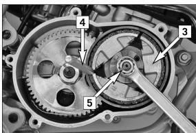
To tune your clutch, lay the bike on the left side. To prevent oil from leaking from the transmission vent hose, run the hose upwards and fasten. Remove the screws [1] and the clutch cover [2] and discard the gasket. Block the centrifugal clutch [3] with a suitable driver [4].
