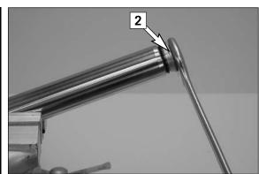
Clamp the fork leg into a vise (use protective jaws) and remove the plugs [2].
