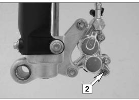
Mount the left brake shoe and fix with screw. Mount the right brake shoe and tighten the screw to 6 Nm. Mount the lock washer. Align brake shoes, mount front wheel (see chapter: Mounting the front wheel).
