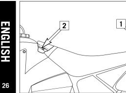
To mount the seat, position seat on the fixing screw [2] and tank, push forward and fix with the quick release.
