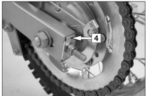
To mount the wheel reverse the procedure described above. Always hook the brake backing plate into the swing arm support. Before tightening the hexagon nut of the wheel spindle, ensure that the supporting plates **[4]** are resting against the swing arm. Additionally, check
