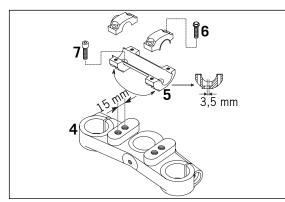
For this purpose, remove screws **[6]** of the handlebar clamps and screws **[7]** of the handlebar support. Position handlebar support, and tighten screws **[7]** to 40 Nm. Mount handlebar and handlebar clamps, and tighten screws **[6]** to 20 Nm. The gap between the handlebar support and handlebar clamps should be the same size in the front and in the rear.
