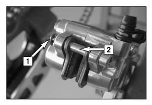
Remove the safety device [1], knock out the guide pin [2] from the brake caliper with a drift towards the chain wheel and remove the brake pads. Carefully clean the brake caliper with compressed air and check the sleeves of the guide pins for damage.
