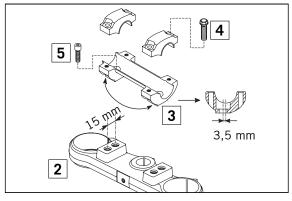
For this purpose, remove screws [4] of the handlebar clamps and screws [5] of the handlebar support. Position handlebar support, and tighten screws [5] to 40 Nm. Mount handlebar and handlebar clamps, and tighten screws [4] to 20 Nm. The gap between the handlebar support and handlebar clamps should be the same size in the front and in the rear.
