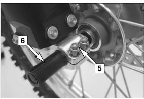
To install the front wheel, lift it into the fork, position and mount the axle shaft. Mount the collar nut [4], tighten the clamping screws [5] on the right fork leg axle passage to prevent the axle shaft from turning and tighten the collar nut to 30 Nm (22,14ft.lb).
