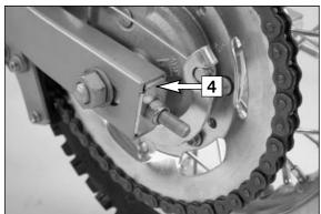
To mount the wheel reverse the procedure described above. Always hook the brake backing plate into the swing arm support. Before tightening the hexagon nut of the wheel spindle, ensure that the supporting plates [A] are resting against the swing arm. Additionally, check
