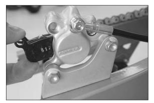
Slide new brake shoes into the brake caliper a fasten with the screw [5]. Tighten the screw to 10 Nm and mount the locking screw [4]. Mount the rear wheel and actuate the foot brake lever until you can feel the pressure point.
