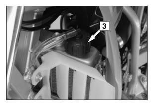
A mixture of 50 % antifreeze and 50 % distilled water is used as the cooling liquid. How-ever, the antifreeze protection must be at least  $-25^{\circ}$  C ( $-13^{\circ}$  F). This mixture offers antifreeze protection but also good corrosion protection and should therefore not be replaced by pure water.
