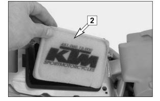
Thoroughly wash the foam filter in special cleaning fluid (Motorex Bio Dirt Remover) and allow it to dry well. Only press out the filter, do not wring it out under any circumstances. Oil the dry foam filter with a high-grade filter oil (Motorex Liquid Bio Power). Also clean the air filter box. Check carburetor collar for damage and that it is filled correctly.
