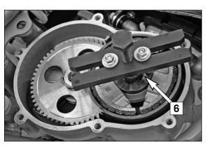
Screw the extractor (special tool item no. 590.29.021.044) onto the clutch hub [6] with the M5x50 screws, hold the extractor and remove the centrifugal clutch from the crankshaft by screwing in the extractor screw. Completely remove the centrifugal clutch, bearings and spacing washers from the crankshaft.
