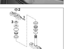
At least once a year, the steering head bearings should be smeared with waterproof grease (Motorex Long Term 2000).
