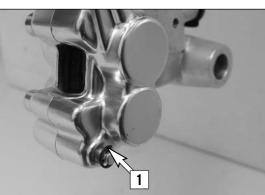
Remove the lock washer [1] from the screw as well as fixing screw [2] and take the brake shoes out of the brake caliper. Clean brake caliper thoroughly with compressed air.
