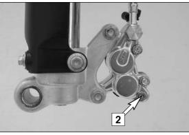
2 Mount the left brake shoe and fix with screw. Mount the right brake shoe and tighten the screw to 6 Nm. Mount the lock washer. Align brake shoes, mount front wheel (see chapter: Mounting the front wheel).
