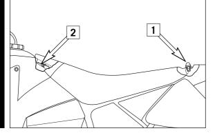
To mount the seat, position seat on the fixing screw [2] and tank, push forward and fix with the quick release.
