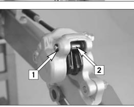
Remove the locking screw [1], unscrew the screw [2] and pull the brake shoes out of the brake caliper.
