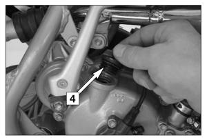
Remove the filler plug **[4]** and add 0.50 l gear oil 20W30 (e.g. Motorex Top Speed 4T 15W50). Mount the filler plug and check the engine for leaks.
