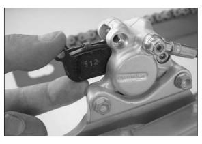
Slide new brake shoes into the brake caliper a fasten with the screw [2]. Tighten the screw to 4 Nm and mount the locking screw [1]. Mount the rear wheel and actuate the foot brake lever until you can feel the pressure point.
