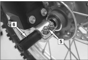
To install the front wheel, lift it into the fork, position and mount the axle shaft. Mount the collar nut [4], tighten the clamping screws [5] on the right fork leg axle passage to prevent the axle shaft from turning and tighten the collar nut to 40 Nm (29,52ft.lb).
